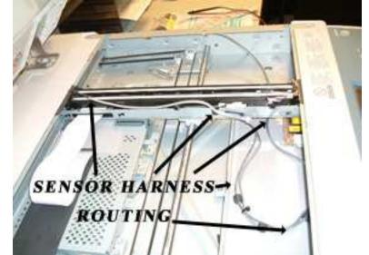
Please note there is plenty of slack in the cable to allow for smooth operation of the scanner light bar. Also note the sensor harness runs UNDER the light bar to exit the copier. Here is a photo of the harness routing on a Samsung C8380ND
